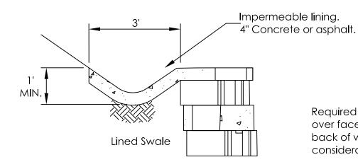
Required to divert surface runoff from flowing over face of wall, to divert water away from back of wall area, and for safety considerations.
